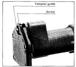
Fix the templet to the workpiece. Move the tool with the templet guide sliding along the side of the templet.
